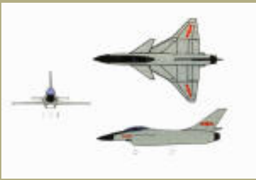
A three-way diagram of the J-10 depicting a compound delta wing
