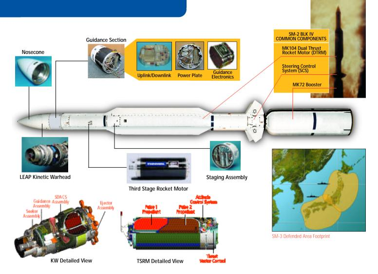
velocity during the exo-atmospheric midcourse phase. The GPS-Aided Inertial Navigation System (GAINS) in the guidance section accurately guides the missile on an intercept trajectory. During flyout, the missile can receive in-flight target updates from the ship to further improve its trajectory. The two-pulse motor design and integral Attitude Control System provide mission flexibility.
