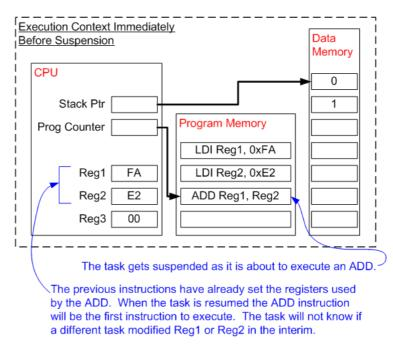
While the task is suspended other tasks will execute and may modify the processor register values. Upon resumption the task will not know that the processor registers have been altered - if it used the modified values the summation would result in an incorrect value.
