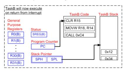
The RTOS tick interrupt interrupted **TaskA**, but is returning to **TaskB** - the context switch is complete!
