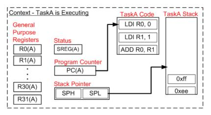
The (A) label within each register shows that the register contains the correct value for the context of task A.
