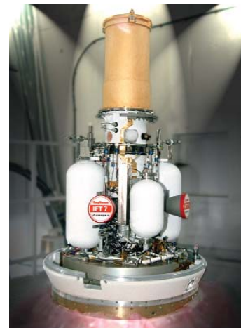
EKV hardware together with the adapter assembly is pictured on the missile access stand at Meck Island in the Marshall Islands.
